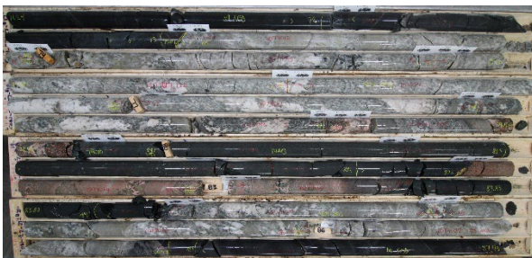
Figure 4C. Spodumene bearing Lithium Pegmatite intersections in drill hole CON-22-27 (Core Interval from 71 to 88 m)
